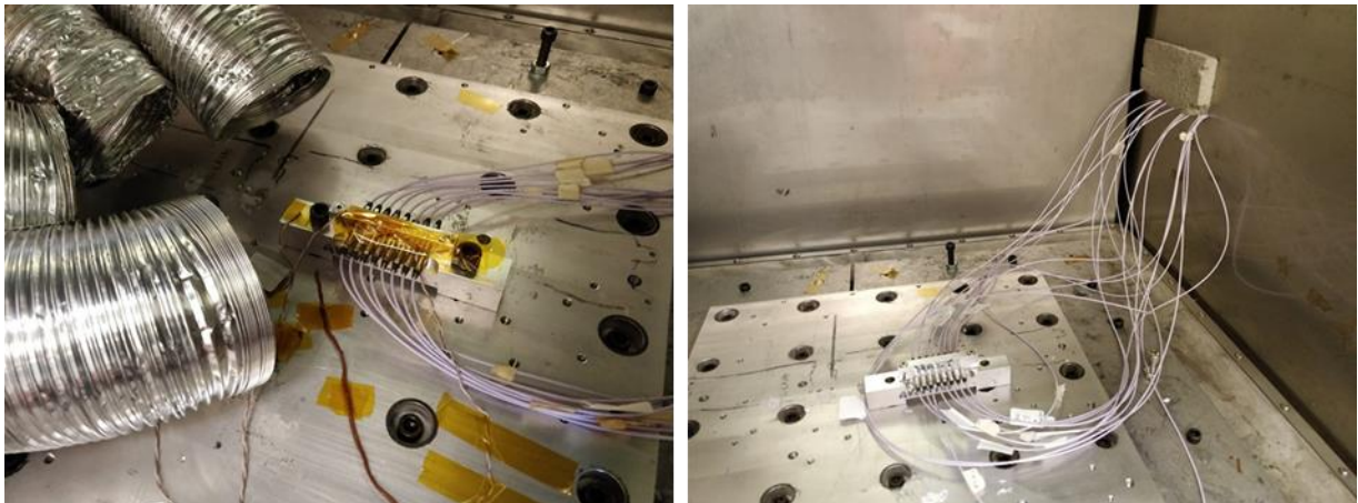
FIGURE 1 HALT TEST SET-UP SHOWING SAMPLES MOUNTED ON VIBRATION BED IN TEST CHAMBER
