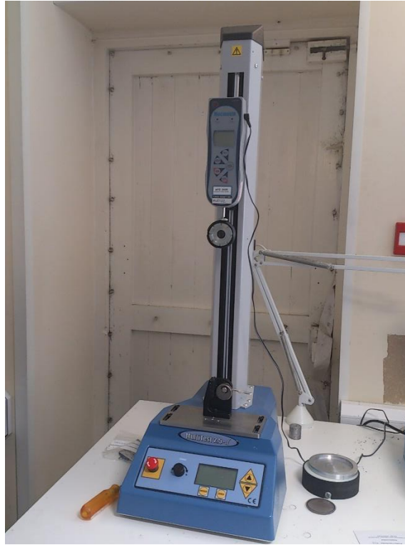
FIGURE 8 TENSILE TEST MACHINE USED TO MEASURE BOND STRENGTH OF CABLE TO SPLICE TERMINUS.
